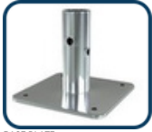
BASE PLATE Standard: EN74 / BS1139 Size: 150mm x 150mm x 6mm Finish: HDG
